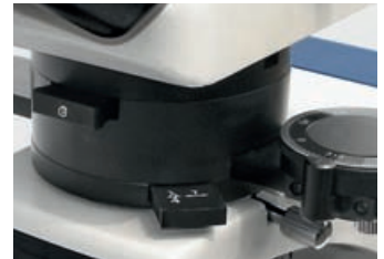
Bertrand lens, \lambda Slip, 360° rotatable analyser (detachable)
