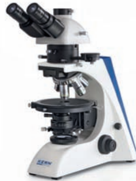
Bertrand lens, \lambda Slip, 360° rotatable analyser (detachable)
